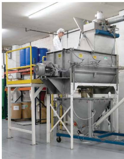
The ribbon blender is fed through a bag dump station and discharges to a floor hopper before blending.
